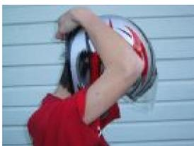
*An essential test before buying or using a helmet, is the roll-off test. With the strap securely fastened, grab the rear lip of the helmet and try to roll it forward off your head. Don't stop just because it hurts a bit. If it comes off, you need a different helmet.* Photo by Art Friedman
