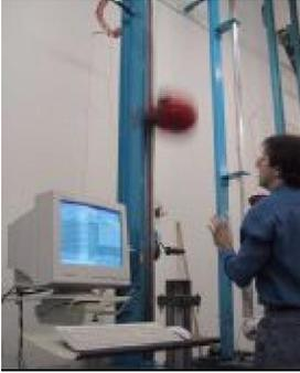
*Helmets are tested in facilities such as the Head Protection Research Laboratory shown here. Drop tests with an instrumented head form measure a helmet's ability to absorb energy in a crash. Photo by Art Friedman.*
