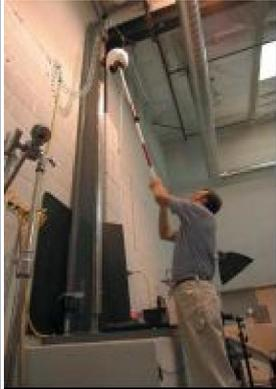
The helmets are mounted on a 5-kilo (11 pound) magnesium headform and then dropped from a controlled height onto a variety of test anvils to simulate crash impacts on various surfaces and shapes. In the real world, your helmet actually hits flat pavement more than 85 percent of the time.
