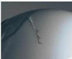
Fiberglass helmets such as the the Arai Tracker (shown) showed substantial damage to their shells after the edge impact. The polycarbonate-shell helmets were largely unmarked. Neither result is essentially better: Either shell material can be used to make excellent helmets. Polycarbonate helmets generally transmit fewer Gs to the head in our testing than fiberglass-shell lids, even when certified to the same standards.
