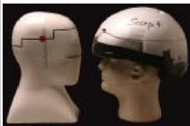
All the Snell/DOT helmets we examined use a dual-density foam liner. The upper cap of foam on this Scorpion liner is softer to compensate for the extra stiffness of the spherical upper shell area. Some manufacturers, including Arai and HJC, use a one-piece liner with two different densities molded together.
