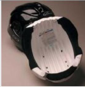
Helmet designers have devised a number of different liner designs to meet the different standards. The Vemar VSR uses stiffer EPS than most, but has channels molded in to soften the assembly (to ECE specs) and enhance cooling.
